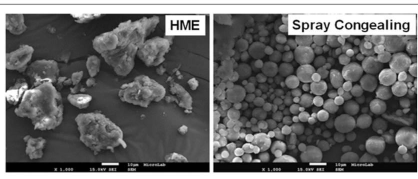
Figure 2. Scanning electron microscopy images of materials produced by two distinct taste masking processes: hot melt extrusion (HME) and spray congealing (SC).
