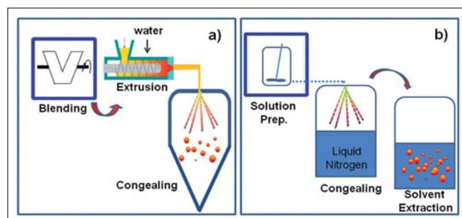
Figure 3. Spray congealing setup: a) combining the feed with and hot melt extrusion process (used in Zmax<sup>®</sup>) and b) spray congealing with cryogenic solvent extraction (used with Nutropin Depo<sup>®</sup>).
