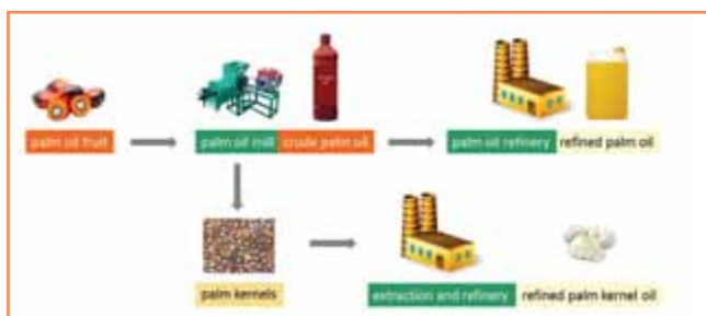
Figure 4. Schematic view of palm oil and palm kernel fat processing.
